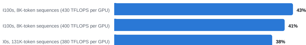
Figure 1. Llama 3 405B pre-training: useful arithmetic per GPU at three cluster configurations (BF16 model FLOPs utilisation)
